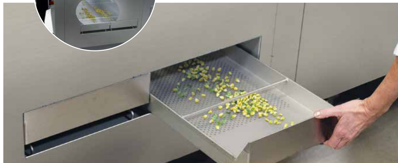
The loading and unloading areas have large strainers, which can be located at either the front or back side of the machine if required.
