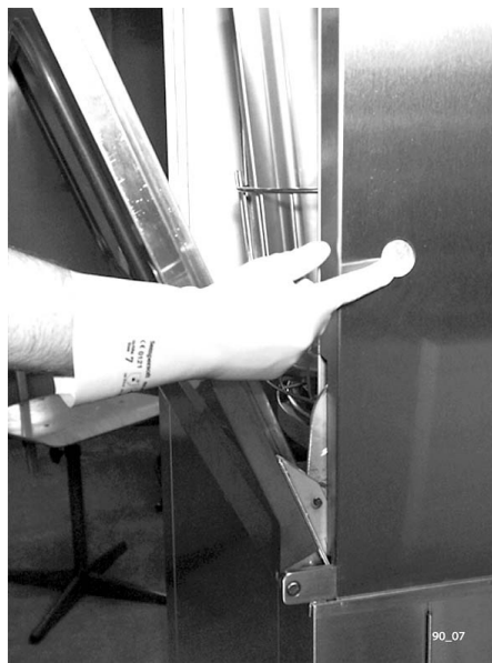
The door pushbuttons (17) for the door lock on the side of the machine.
