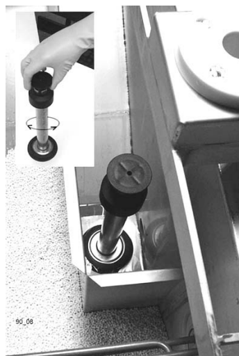
The level pipe (21) and the rubber seal (22).
