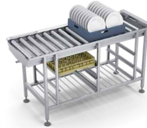
The roller conveyor has a sloping bottom and is equipped with drain towards floor or curve. At the end of the conveyor, the sides are lowered and aligned with the rollers, allowing the baskets to be pulled out without heavy lifting.
