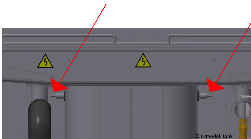
Detergent hose connections on both sides of the tank
